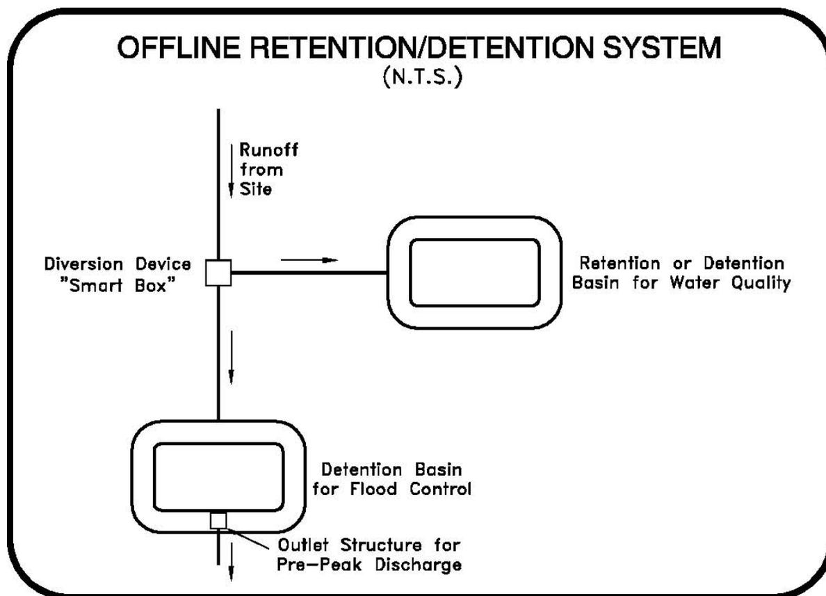
Figure 5-4. Schematic of an Off-Line Retention/Detention System.
