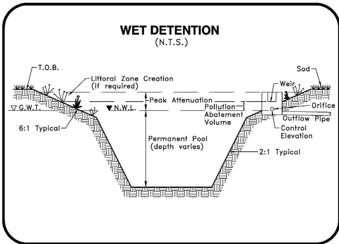
Figure 5-2. Schematic of a Wet Detention System.
