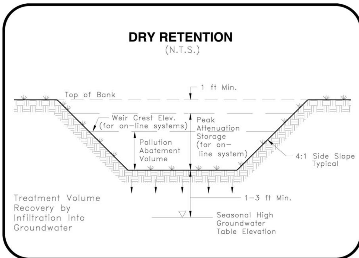
Figure 5-1. Schematic of a Dry Retention Facility.
