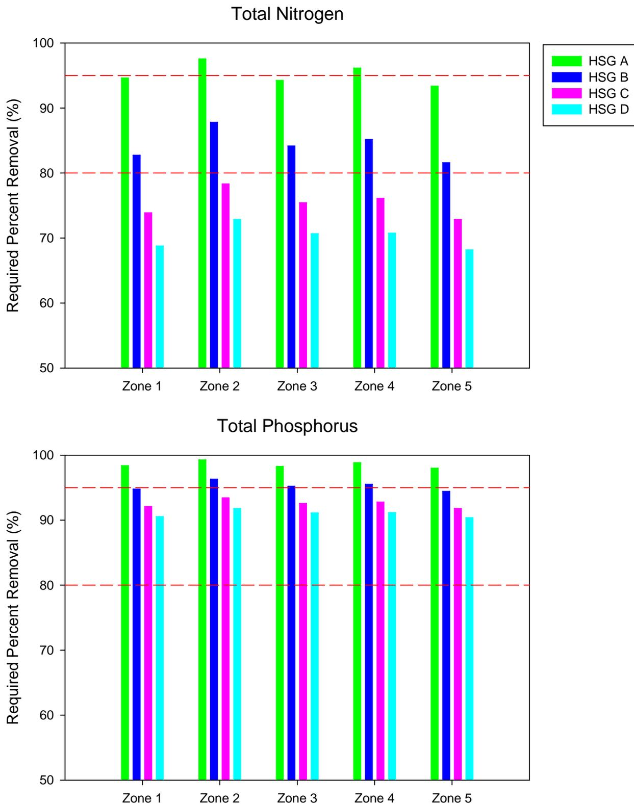
Figure 6-7. Comparison of Estimated Annual Mass Removal Efficiencies to Achieve Post-Development  $\leq$  Pre-Development Loadings of Nitrogen and Phosphorus for a Single-Family (25% Impervious) Residential Development.
