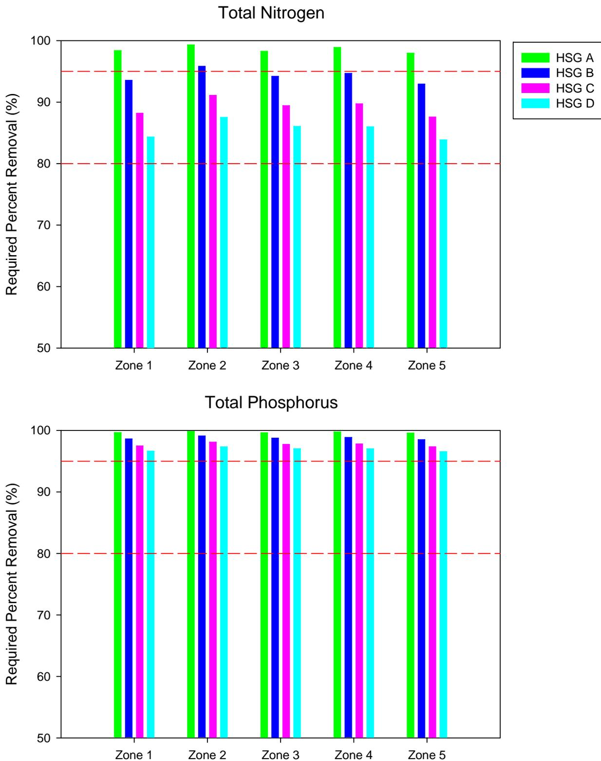
Figure 6-9. Comparison of Estimated Annual Mass Removal Efficiencies to Achieve Post-Development  $\leq$  Pre-Development Loadings of Nitrogen and Phosphorus for a Multi-Family Residential Development.
