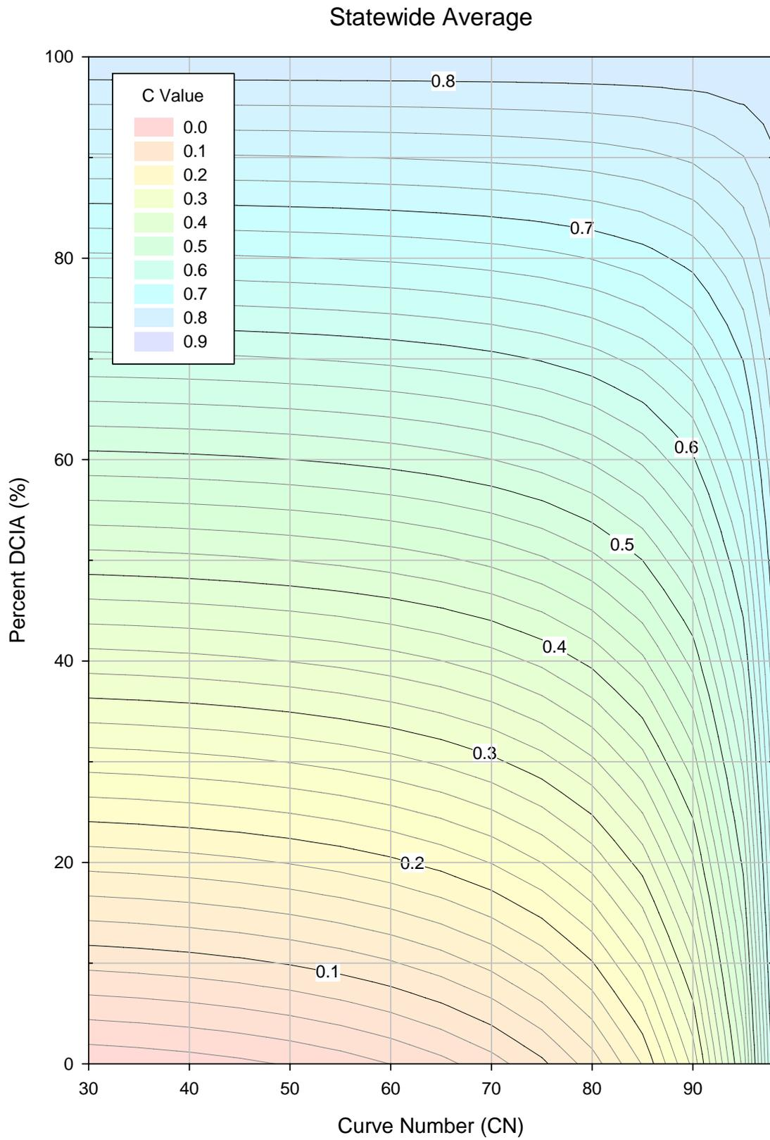
Figure 4-7. State-wide Mean Distribution of C Values as a Function of DCIA and Curve Number.
