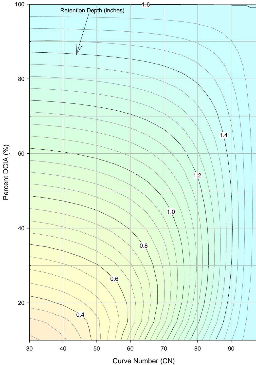
Figure 6-2. State-wide Average Variations in Required Dry Retention Depth for 80% Removal as a Function of DCIA Percentage and non-DCIA Curve Number.
